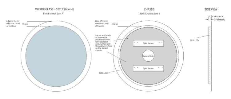
The 'Front Mirror Part A' sides over and locks on to the split battans on 'Back Chassis Part B'
